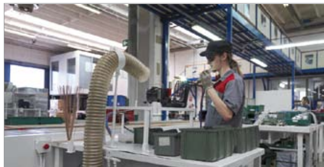
Welding of the condenser to the compressor
